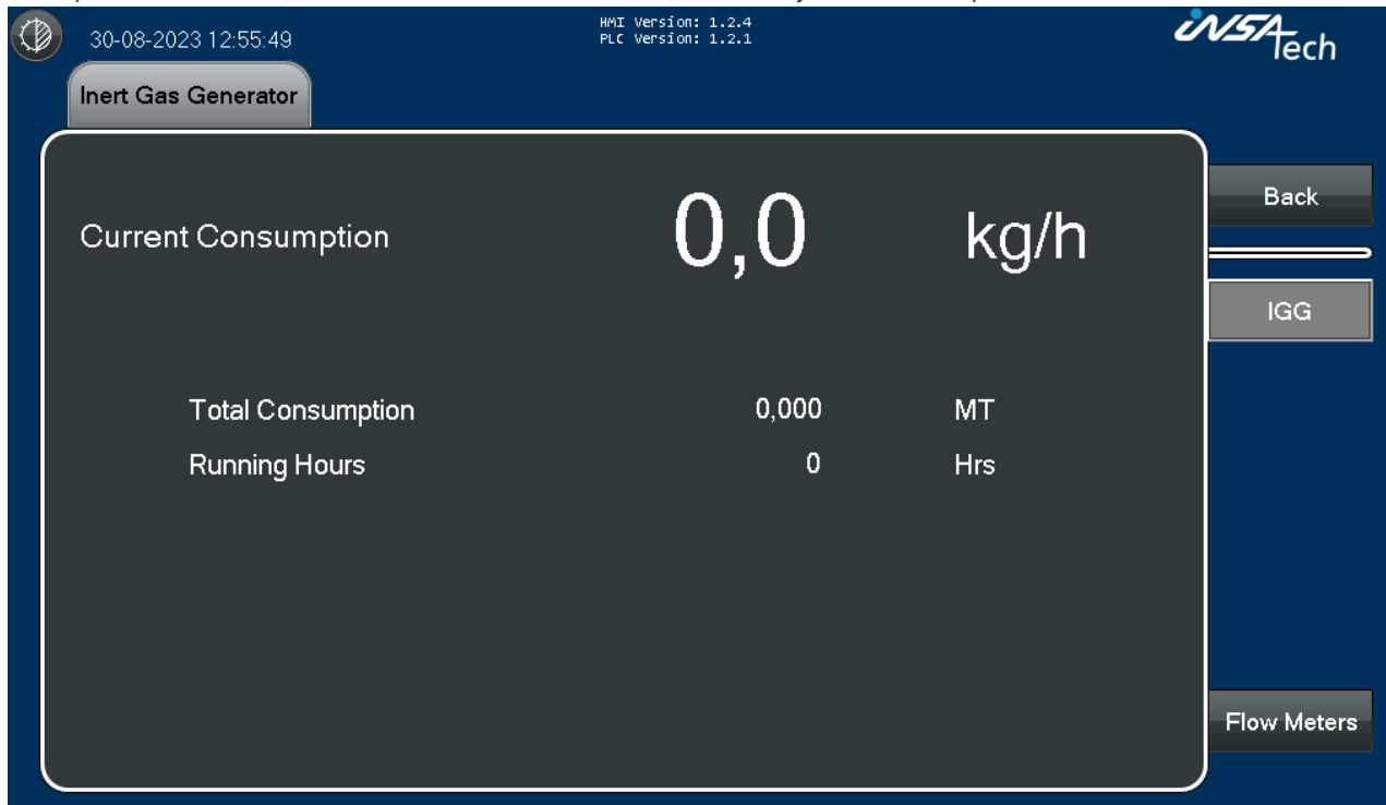
Example of a consumer, in this case Inert Gas Generator, where only Fuel Consumption is measured.
