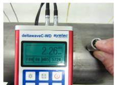
deltawaveC-WD determines the thickness of a structure or a pipe by accurately measuring the time required for a ultrasonic signal to travel through the thickness of the material, reflect from the back or inside surface, and be returned to the transducer. The measured two-way transit time of the ultrasonic together with the specific speed of sound of your material is used to accurately measure the wall thickness. The resolution is 0.1mm
