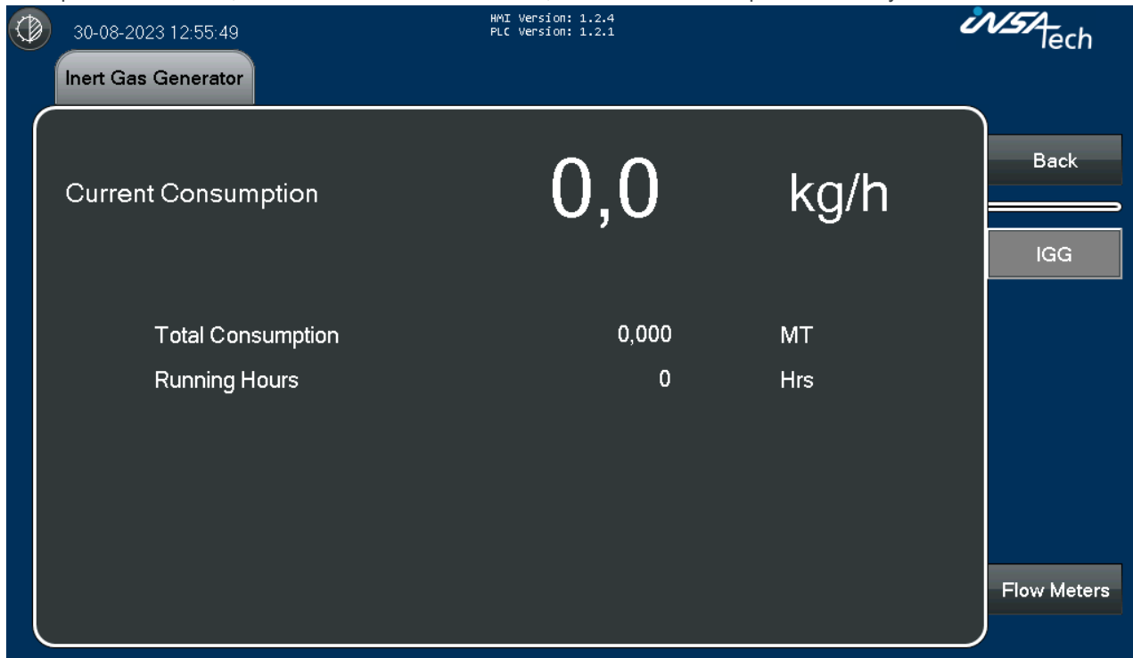
Example of a consumer, in this case Inert Gas Generator, where Fuel Consumption is the only measurement.
