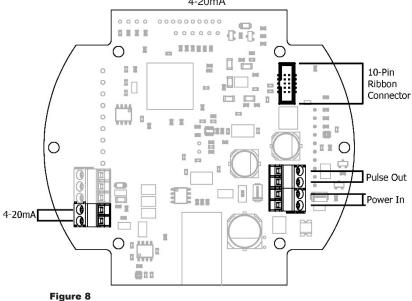
WIRING DIAGRAM Inputs: GPI Custom Sensor Outputs: 4-20mA, Pulse Output
