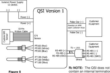
**R2 NOTE:** The QSI does not contain an internal termination resistor. Refer to Customer Equipment documentation for proper installation and resistance value of the external R2 resistor.
