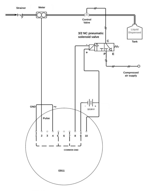
Note: 'PRECLOSE' software setting should be set to zero for single stage batch control
