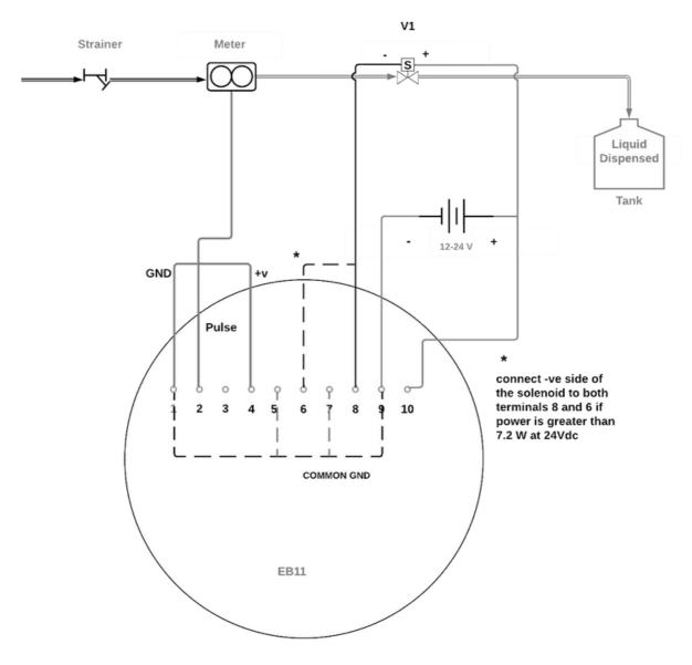
Note: 'PRECLOSE' software setting should be set to zero for single stage batch control
