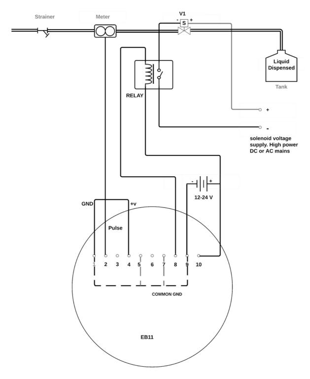
Note: 'PRECLOSE' software setting should be set to zero for single stage batch control
