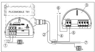
Fig. 10: Connection of the voltage supply
