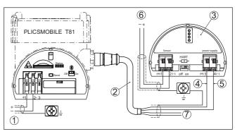
Fig. 8: Connection of the voltage supply and VEGADIS 82 HART
