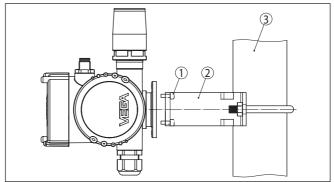
Fig. 4: PLICSMOBILE T81 for tube mounting
