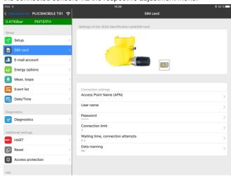
Fig. 16: Example of an app view - Settings SIM card
