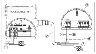
Fig. 6: Connection voltage supply and plics® sensor
