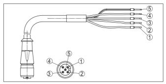
Fig. 9: Connection assignment, sensor connection cable
