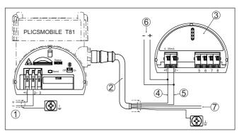
Fig. 11: Connection of the voltage supply
