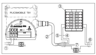
Fig. 7: Connection of the voltage supply and VEGABOX 03
