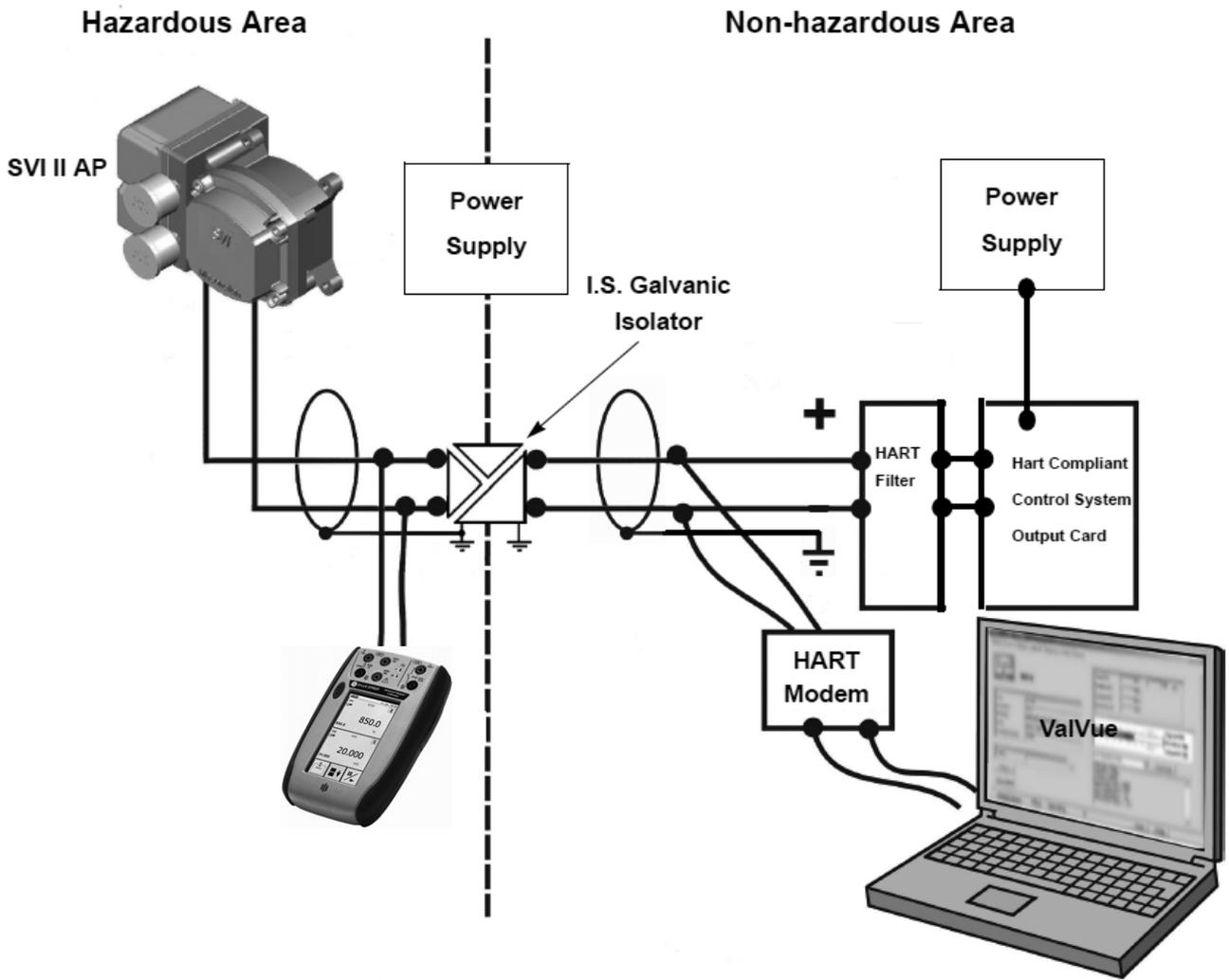
**Figure 47 Intrinsically Safe Installation with Galvanic Isolator**
