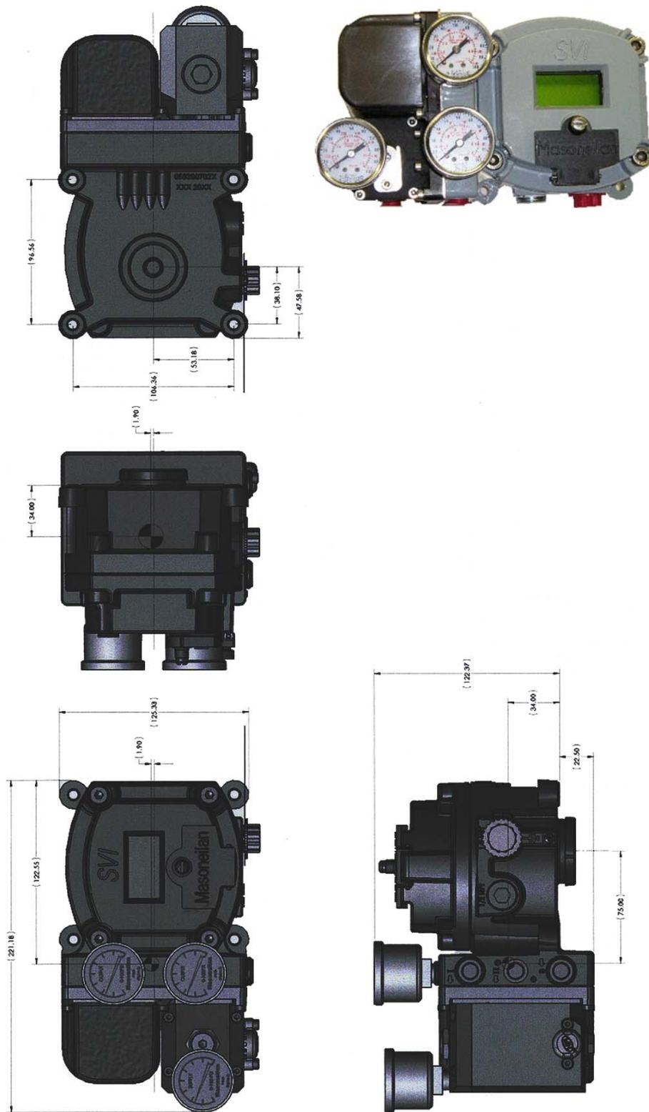
Figure 8 SVI II AP Double-Acting Dimensions
