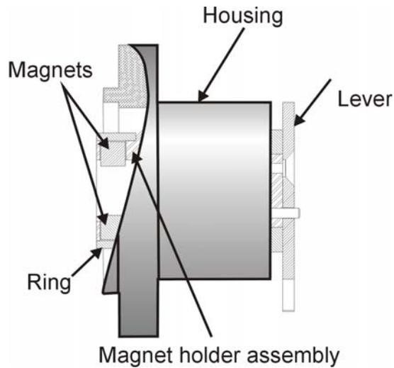
**Figure 14 Magnet Holder for Reciprocating Valves**
