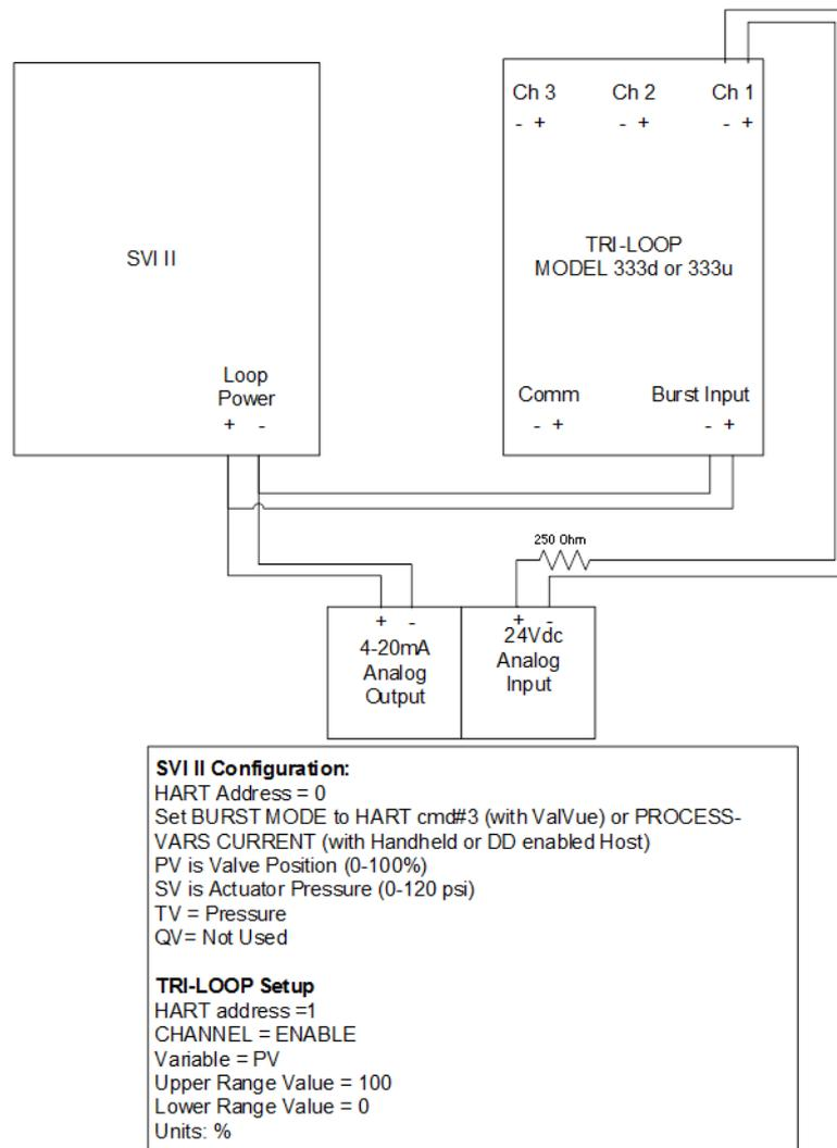
**Figure 71 Sample Tri-Loop Configuration**
