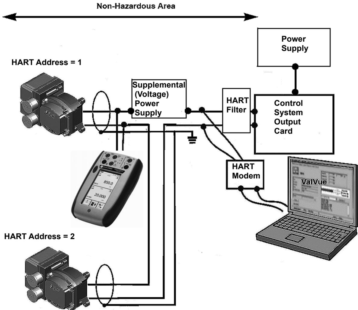
**Figure 45 Split Range with Supplemental Power Supply - Non-Hazardous**
