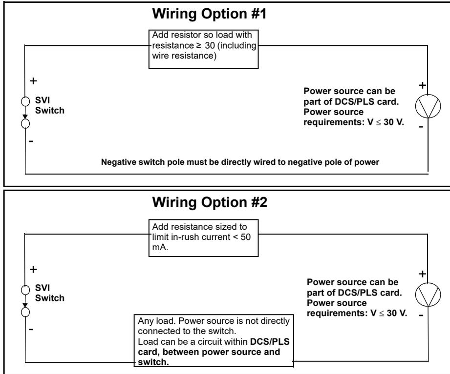
Figure 51 DCS Switches Wiring Options
