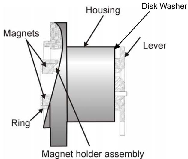
**Figure 29 Magnet Holder for Reciprocating Valves**
