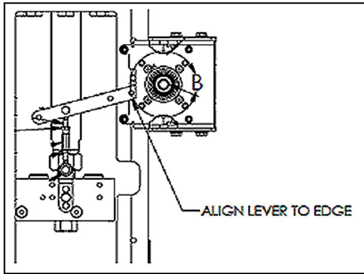
**Figure 22 Lever Alignment**
