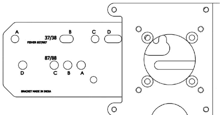
**Figure 30 Reciprocating Valve Mounting Bracket**
