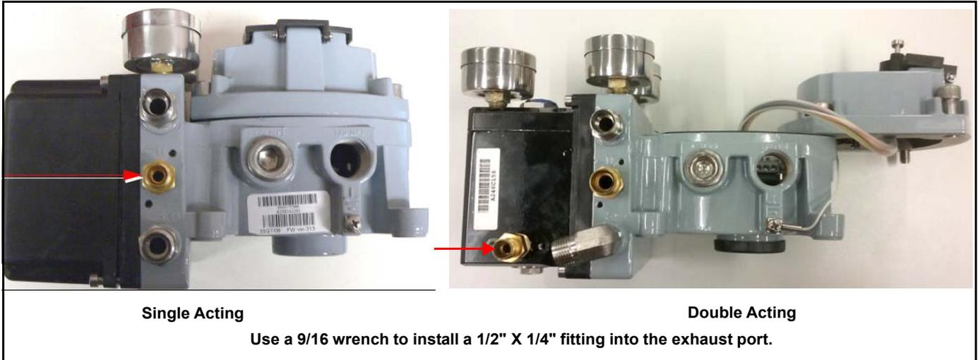
**Figure 66 Step 2 Install a 1/2" x 1/4" Fitting**
