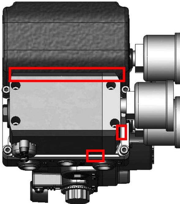
**Figure 56 Bleed Slots on Complete Unit**
