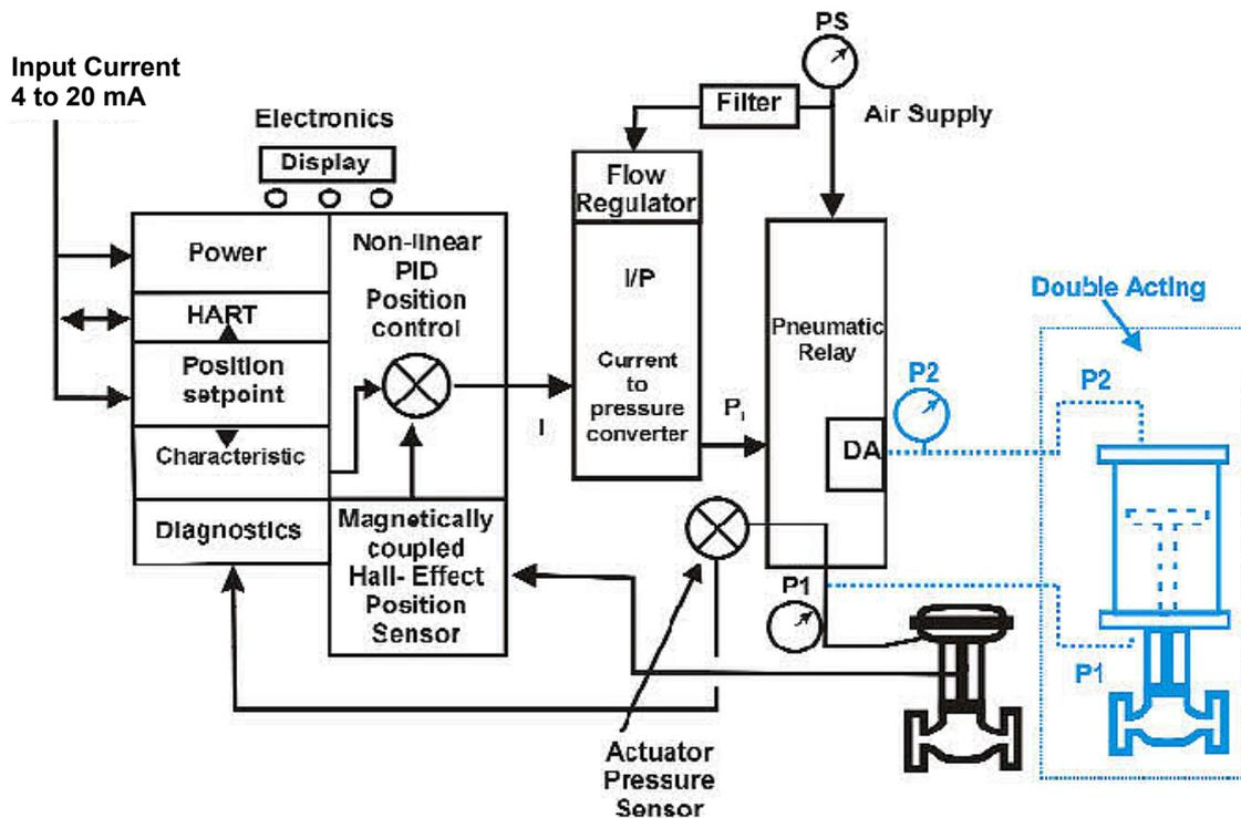
Figure 48 Block Diagram with I/P Converter and Pressure Sensor
