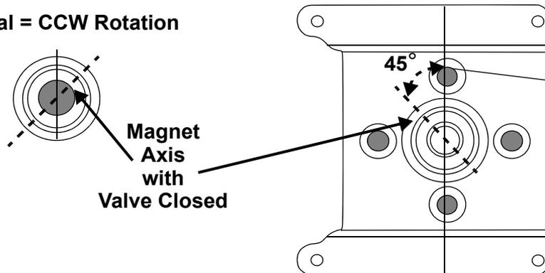
**Figure 28 Magnet Orientation for 90° Valve Rotation with De-energized Actuator**
