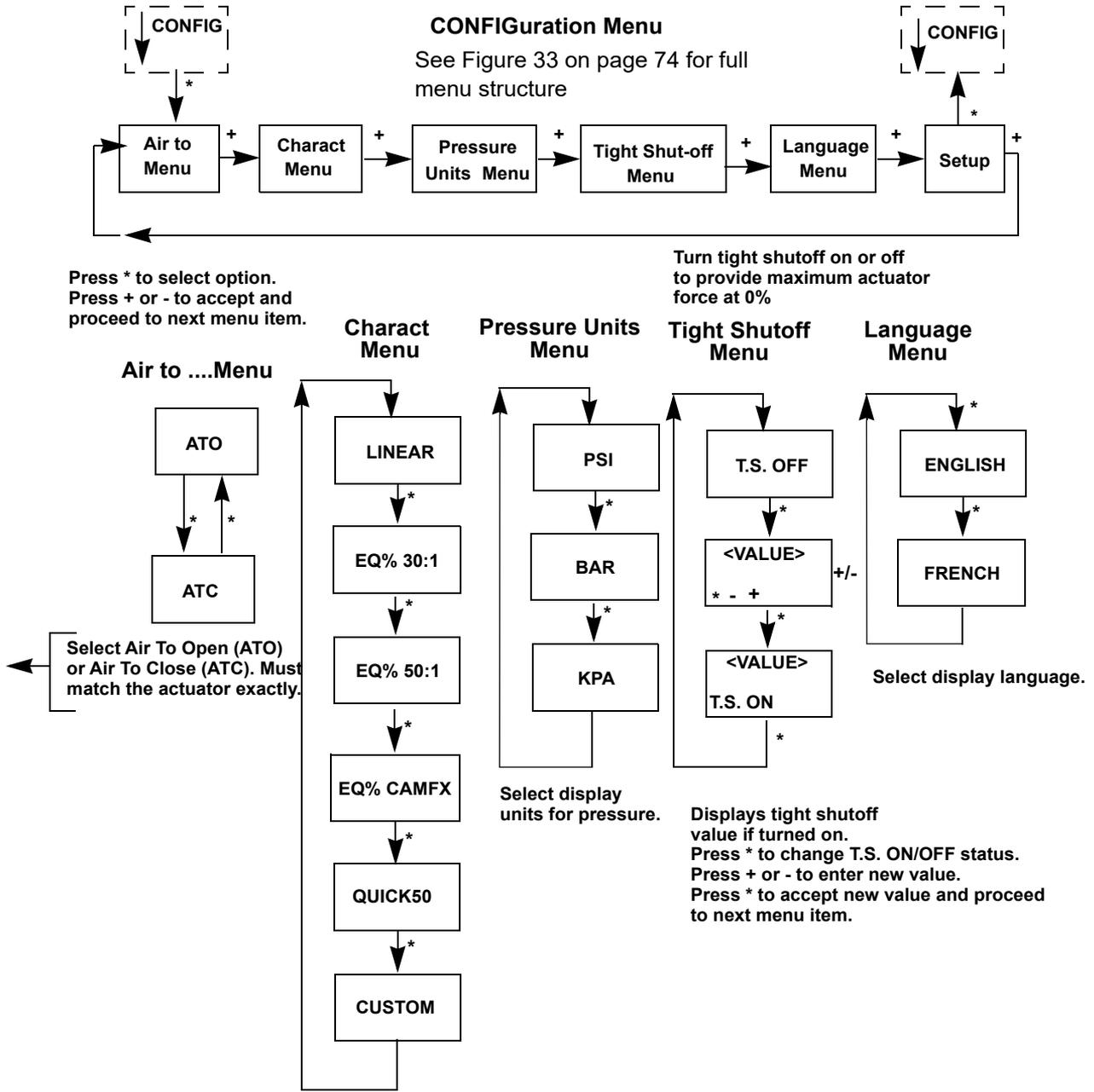
**Figure 39 Configuration Pushbutton Guide**
