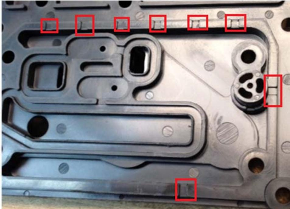
**Figure 55 Bleed Slots On Air Routing Plate**
