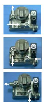
Shown above, each of the inlet & outlet valve assemblies may be repositioned in one of three 90 degree incremental positions by accessing the socket head screws on the underside of the manifold.
