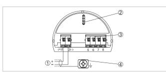
Secondary terminal connections (intrinsically safe devices)
