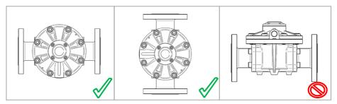
Liquid can flow in a horizontal direction, or a vertical direction, but in each case the rotor shafts must be in a horizontal plane. This is achieved by mounting the meter so that the terminal cover, or integral instrument display, is facing in a horizontal direction. For pulse output flowmeters the direction of flow is not important, as the output is non-directional.
