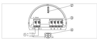
Electronics and terminal compartment, single chamber housing
