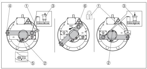
Fig. 31: Switching the radiation on - VEGASOURCE 31 version B
