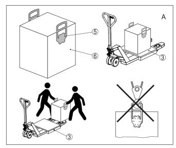
Fig. 10: Transport of the type A packaging
