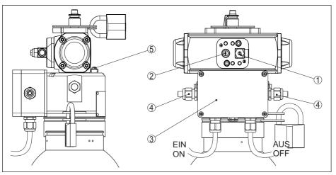
Fig. 27: Connection of the pneumatic lines on VEGASOURCE 31 - version K. M.
