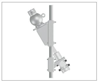
Fig. 18: 30° measurement setup on a pipeline with diameter 50  $\dots$  100 mm (1.97  $\dots$  3.94 in)
