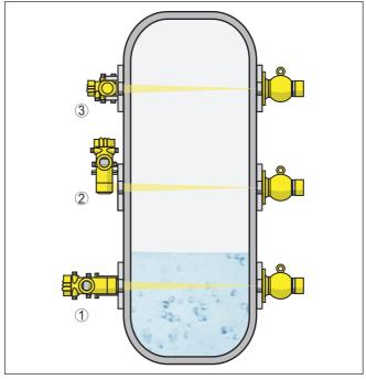
Fig. 16: Installation positions - Point level detection with MINITRAC 31
