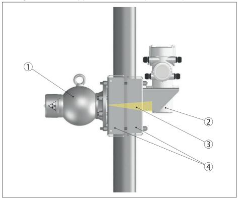
Fig. 57: Mounting brackets for mounting on pipes from 50  $\dots$  220 mm (1.97  $\dots$  8.66 in) for 30° diagonal irradiation
