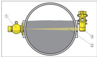
Fig. 21: Measurement setup on a horizontal pipeline
