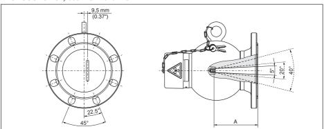
Fig. 53: Beam exit channel (e.g. version A)
