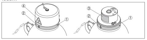
Fig. 3: Position of the type labels - Version A
