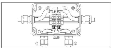
Fig. 29: Connection terminal housing of the position indicators
