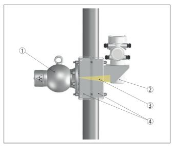
Fig. 19: Measurement setup on a pipeline with a diameter of 50 ... 420 mm (1.97 ... 16.54 in), detector mounting vertical
