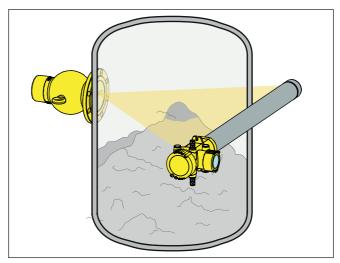
Fig. 17: Point Level detection with SOLITRAC 31
