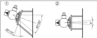
Fig. 22: Correct mounting of the fire-proof version
