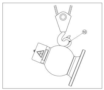
Fig. 13: Crane transport of the source holder 10 Luq
