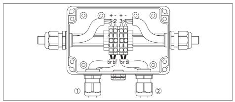
Fig. 26: Connection terminal housing of the proximity switches
