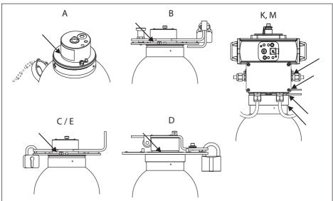
Fig. 37: Wiping surfaces for the tightness test
