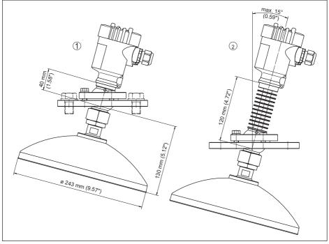
Fig. 64: VEGAPULS SR 68, parabolic antenna and swivelling holder
