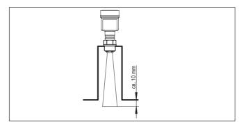
Fig. 8: Recommended socket mounting with horn antenna
