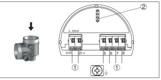
Fig. 27: Electronics compartment - double chamber housing
