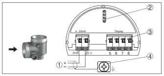
Fig. 28: Connection compartment - double chamber housing
