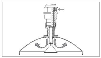
Fig. 24: Purging air connection with parabolic antenna
