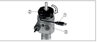
Fig. 41: Connection of the PC directly to the sensor via the interface adapter
