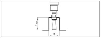
Fig. 12: Deviating socket dimensions
