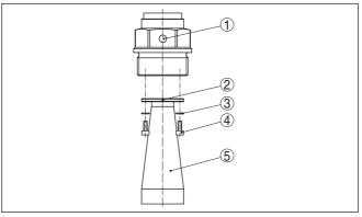
Fig. 2: Dismounting of the horn antenna
