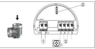
Fig. 30: Electronics compartment - Ex-d-ia double chamber housing
