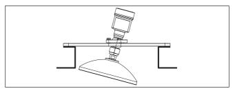
Fig. 11: Distance between antenna and socket with parabolic antenna
