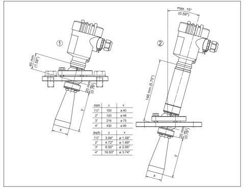
Fig. 63: VEGAPULS SR 68, horn antenna and swivelling holder
