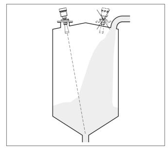
Fig. 6: Mounting of the radar sensor with inflowing medium
