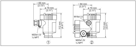
Fig. 56: Housing versions in protection IP 66/IP 67 (with integrated display and adjustment module the housing is 9 mm/0.35 in higher)
