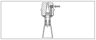
Fig. 23: Purging air connection with horn antenna
