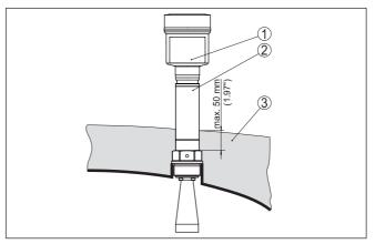
Fig. 19: Mounting the instrument on insulated vessels.
