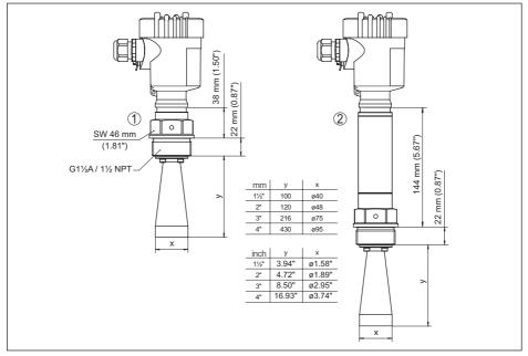
Fig. 61: VEGAPULS SR 68, horn antenna in threaded version
