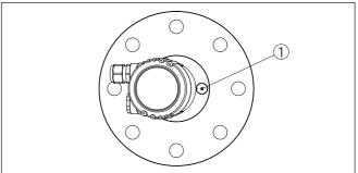
Fig. 15: VEGAPULS SR 68 with swivelling holder
