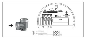
Fig. 29: Connection compartment - Radio module PLICSMOBILE 81
