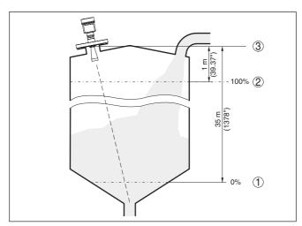
Fig. 40: Parameterisation example, Min./max. adjustment
