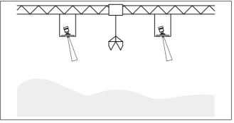
Fig. 18: Radar sensors on traverse crane
