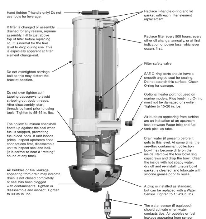
may indicate it is loose or O-ring is damaged. Tighten to 15-20 in. lbs.
