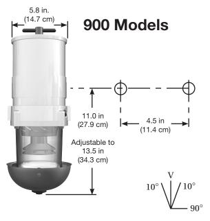
Note: Mount filter assembly as close to vertical (V) as possible. Do not exceed 10° from vertical or assembly may not function properly. Fastener size is 3/8" (M10) for mounting brackets.
