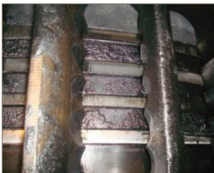
Deposit build up on piston due to over lubrication (too high feedrate)
