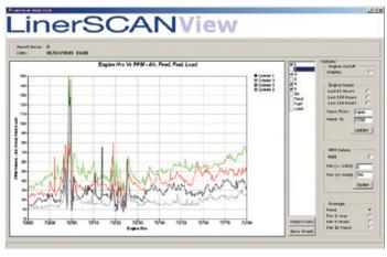
An 'Overview' tab shows all readings, an event log and allows exporting of the data and log information which can be sent to the head office for further investigation if needed.
