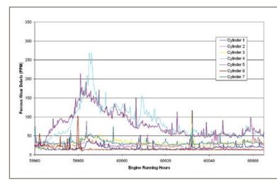
This chart shows the ability of LinerSCAN to detect and trend the amount of iron particles in the cylinder oil in real time.
