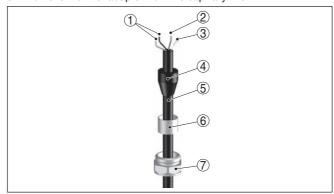
Fig. 15: Configuration of the cable seal
