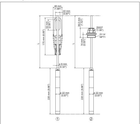
Fig. 16: VEGAWELL 52, with transmitter 316L/Titanium 22 mm
