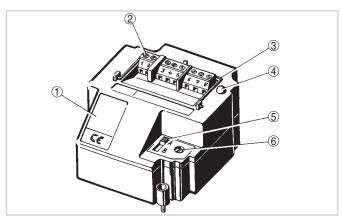
Oscillator with relay output
