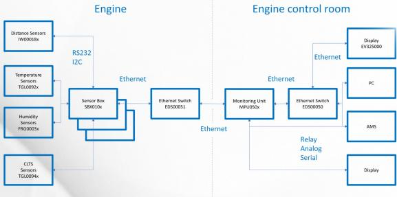
The distance, temperature as well as the water in oil values are read by the **sensor box SBX010x** and are then transferred over ethernet to the **monitoring unit MPU050x**.
