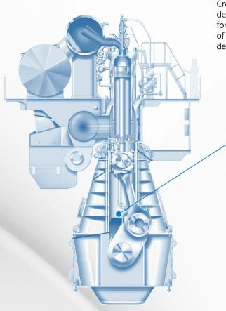
Crosshead position control in lower dead end. Double sensor alignment for monitoring straight movement of crosshead. Each sensor with detection range of 4mm.
