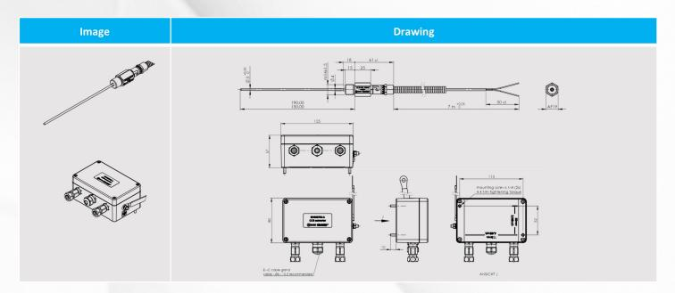
Internal spring force pushes the sensor tip to the surface of the bearing to be controlled.
