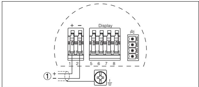
Fig. 11: Wiring plan - single chamber housing
