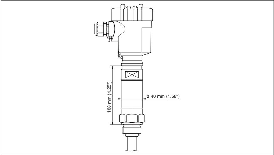
Fig. 38: Temperature adapter
