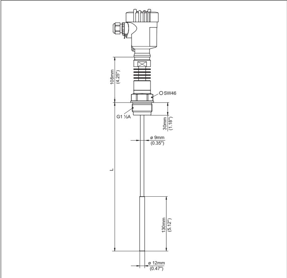
Fig. 37: VEGACAL 65, PTFE-insulated cable ( $\varnothing 8 \text{ mm}$ ) with crimping sleeve /  $-50 \dots +200 \text{ }^\circ\text{C}$
