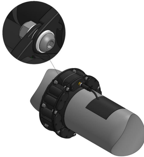
Figure 15 - Pivot Bolts Tightening
