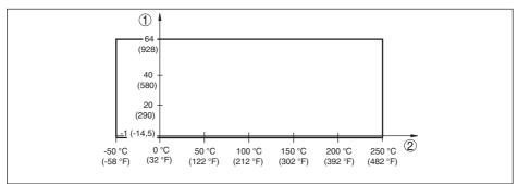
Fig. 16: Process temperature - Process pressure with switch position  $\geq 0.7$  g/cm<sup>3</sup> (sensitivity switch)
