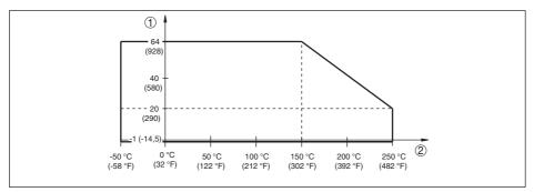
Fig. 17: Process temperature - Process pressure with switch position  $\geq$  0.5 g/cm<sup>3</sup> (sensitivity switch)
