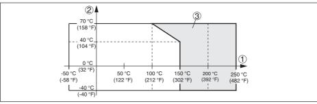
Fig. 15: Ambient temperature - Process temperature
