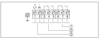
Fig. 10: Wiring plan, single chamber housing
