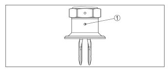
Fig. 7: Marking on the welded socket
