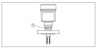
Fig. 5: Fork position with flange versions
