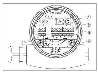
Fig. 9: Electronics and connection compartment, single chamber housing
