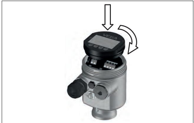
Fig. 43: Installing the display and adjustment module in the electronics compartment of the single chamber housing
