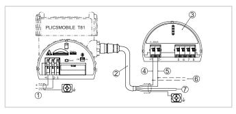
Connection of the voltage supply in the electronics housing
