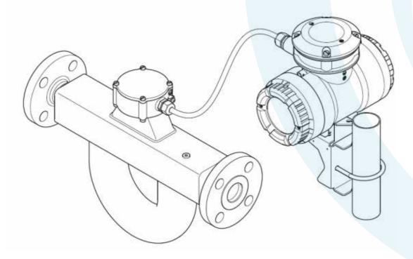
At zero flow, the oscillation of the 'legs' will be synchronized with both sensors registering the same pulse frequencies at the same time. When a flow is introduced through the sensor piping, the U-shaped sensor pipe will start to 'wiggle' due to the Coriolis Effect, as the moving mass will 'delay' the upstream pulse. The two sensors will now experience an offset in the pulses, and the larger the offset the larger the flow is.
