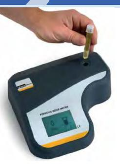
To perform the test just add 5 ml of oil sample to the tube and place it in the test chamber of the unit. The metallic content of the sample will be shown in ppm on the LCD screen in less than 2 seconds.
