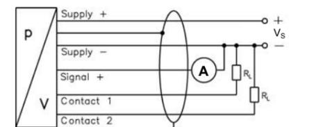
**📖** For the electrical connection a shielded and twisted multicore cable is recommended.
