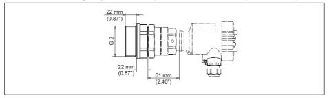
Fig. 12: Mounting adapter with ceramic cover (optional) for VEGAMIP 61 with internal horn antenna, threaded version G1½ with PTFE cover (also with 1½ NPT thread)
