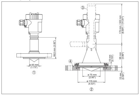
Fig. 10: VEGAMIP 61, encapsulated antennas
