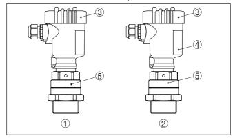
Fig. 1: VEGAMIP 61 with plastic housing
