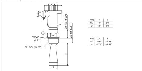
Fig. 11: VEGAMIP 61, horn antenna/316L
