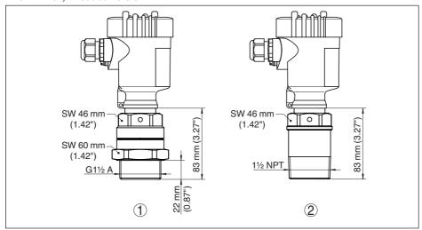
Fig. 9: VEGAMIP 61, internal horn antenna (threaded version)
