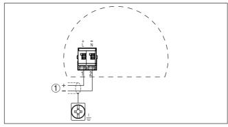
Fig. 7: Wiring plan emitting unit - VEGAMIP 61 (transmitter)
