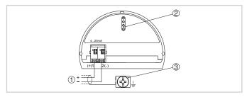
Electronics and terminal compartment, single chamber housing
