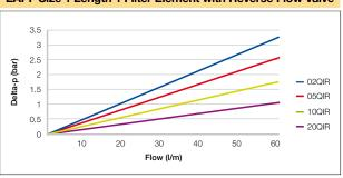
EAPF Size 1 Length 2 Filter Element with Reverse Flow Valve
