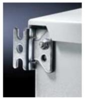
For fast, time saving installation of the indicator box, use wall mounting brackets. Simply insert the expandable dowel into the hole on the backside of the box from the outside and screw-fasten the wall bracket from the outside. In this way the wall bracket securely can by tighten without opening the box door.
