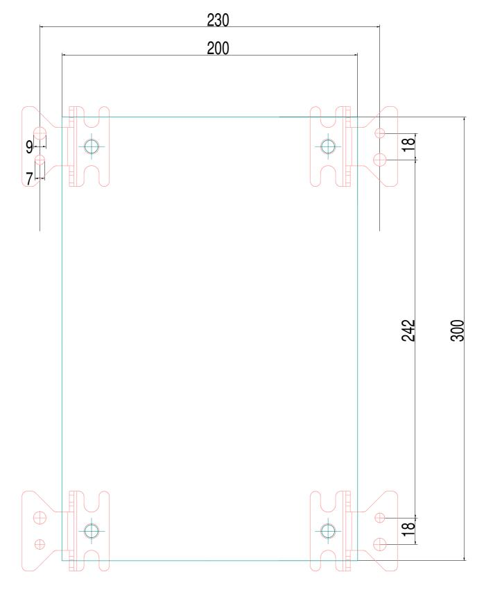
Fixing and mounting sizes [mm] of Indicator Box
