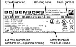
Fig. 1: Example of manufacturing label
