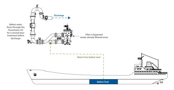
Purestream system is validated to operate at **minimum** retention times (≤ 24 hours) following treatment of 100% of the maximum flow under difficult water conditions with UV transmittance as low as **40% UVT**.
