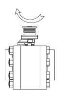
Turn the valve handle  $90^{\circ}$  LD housing to the close position
