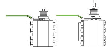
Valve locked in open possition
