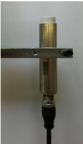
Fig. 38a: sensor with straight connectors
