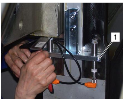
Fig. 42: Adjusting second sensor
