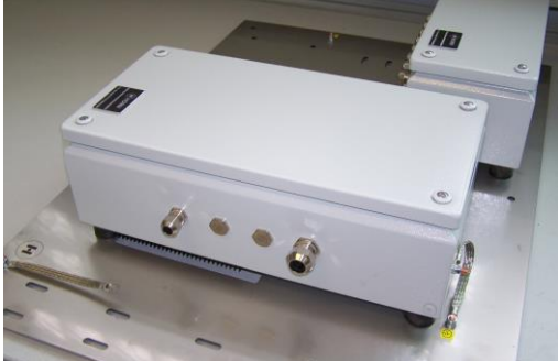
Fig. 11: Line Converter box closed
