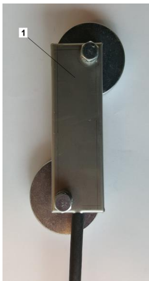
Fig. 5: Splash oil temperature sensor
