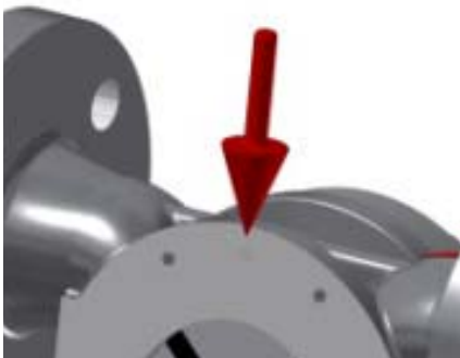
Figure 38 – Damage caused by jacking bolts
