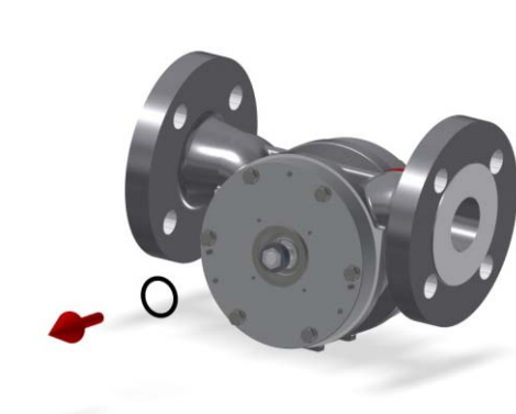
Figure 23 – Remove the O-ring
