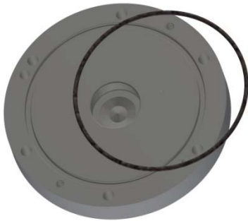
Figure 45 – O-ring on the back cover
