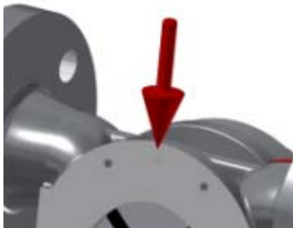
Figure 31 – Damage caused by jacking bolts
