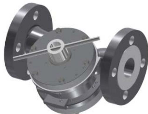
Figure 60 – Tightening the nut of the magnet cap
