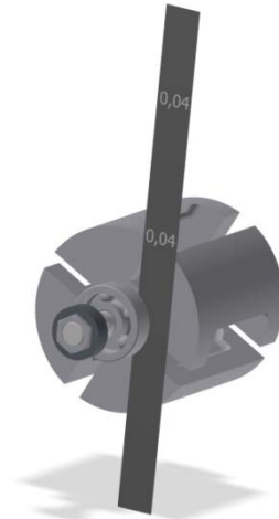
Figure 40 – Measuring the clearance between the vane and the vane slot. (J5025E, J5040E and J5050E)
