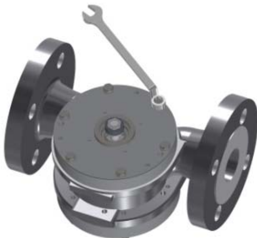
Figure 54 – Installing the front cover
