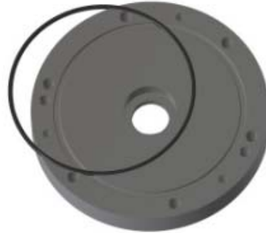
Figure 30 – O-ring on the front cover
