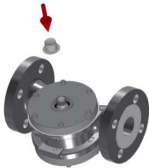
Figure 58 – Installing the magnet cap
