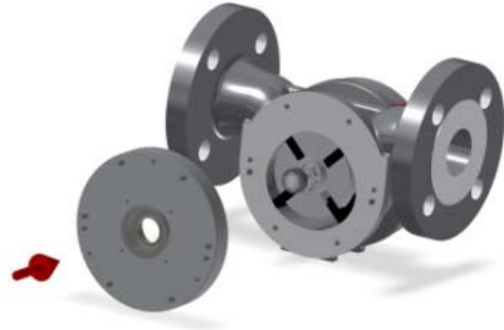
Figure 53 – Positioning the front cover and installing it
