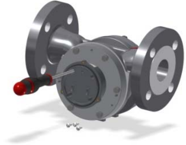
Figure 62 – Install the holder using the 4 bolts
