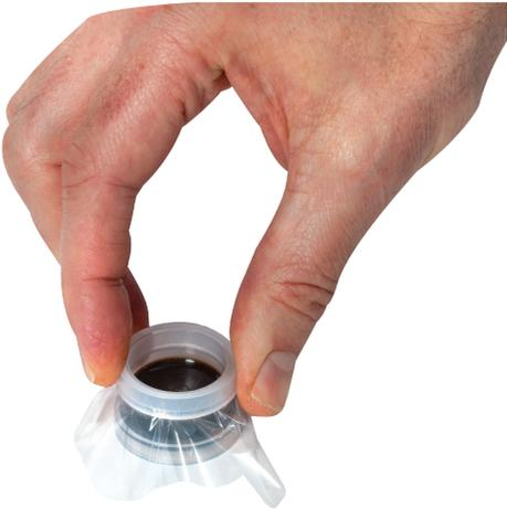
At this stage the sample cup can be safely inverted in preparation for insertion into the XRF Analyser.
