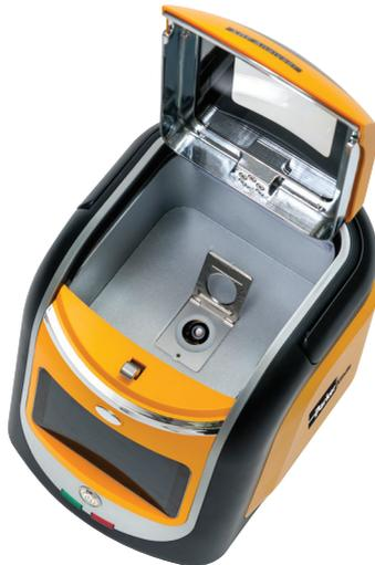
Carefully remove the existing Mylar sheet from over the detector window.
