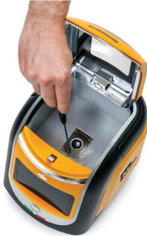
Lift front end of retaining plate using a small screwdriver and hinge backwards.
