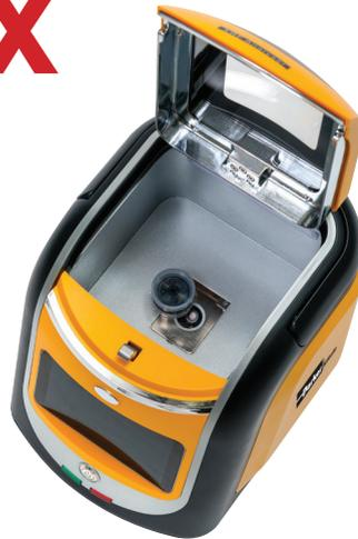
Press the FUEL button on the HOME screen if you wish to determine the sulphur content in a fuel or the LUBE button if you wish to determine the wear metal content in a lubricant. The unit will present a START screen.
