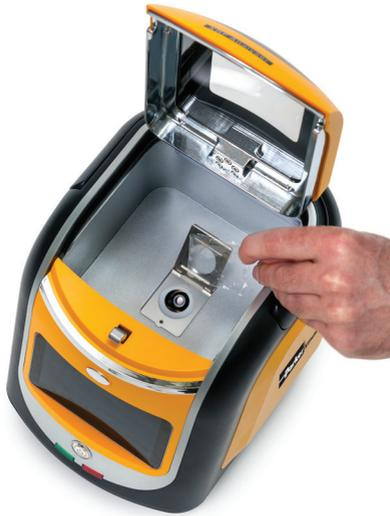
Cut a square of Mylar film from the roll provided and rest it gently over the aperture.
