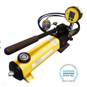
The **PCA205M** - digital pressure calibrator is a microprocessorcontrolled, accurate and versatile digital pressure measuring and calibration instrument with integrated fast peak-, max.- and min.- function. Hydraulic test pressure is generated by the integrated hydraulic pump while read out is done on the digital indicator.
