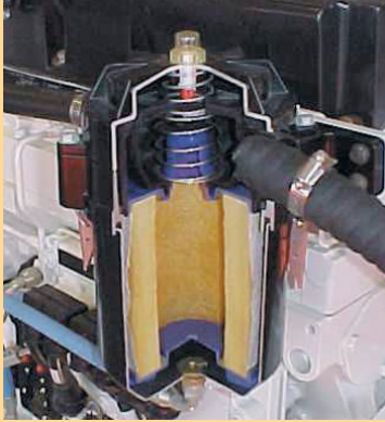
Cummins QSM11 marine engine with CCV cutaway
