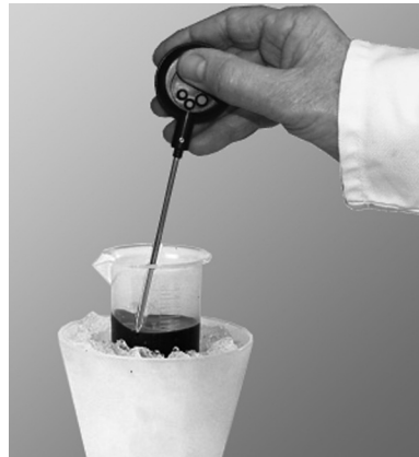
Insert the thermometer and take the temperature of the oil in the beaker.
