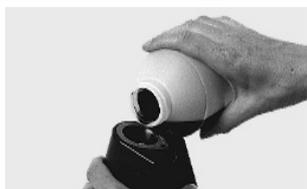
Fill the tube with oil to just above the edge of the V-plate.
