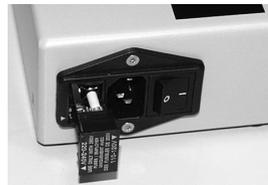
Replace box, ensuring white arrows are aligned to correct voltage supply.
