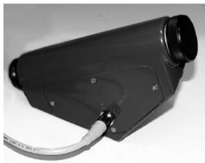
Connect lead to viscometer.
