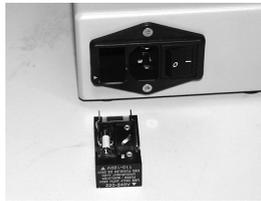
Fit 2 correct fuses for voltage.
