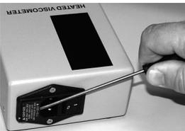
Remove fuse box using a screwdriver.
