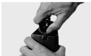
Slacken bleed valve and remove end plug.
