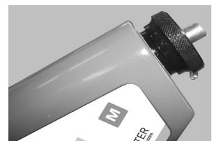
Slowly push in and rotate the end cap until all air is expelled. Tighten the bleed valve.
