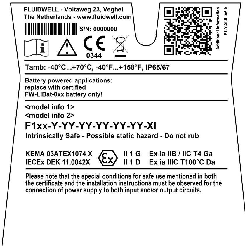
Fig. 25: Label information - Intrinsically safe application (typical)
