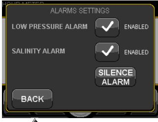
Figure 3.11: Alarms configuration screen.
