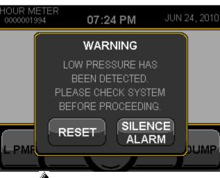
Figure 3.5: Low pressure warning window.
