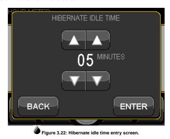
Pressing the arrow <u>UP</u> and <u>DOWN</u> buttons will increment and decrement, respectively. Pressing the <u>BACK</u> button will cancel any changes, while pressing the <u>ENTER</u> button will save any changes.
