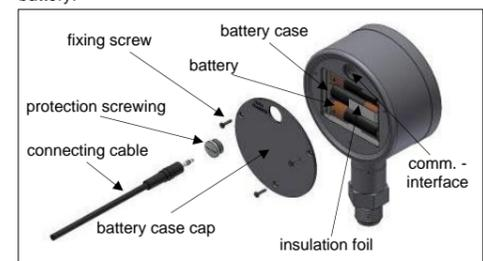
Fig. 3 Battery case and communication interface
