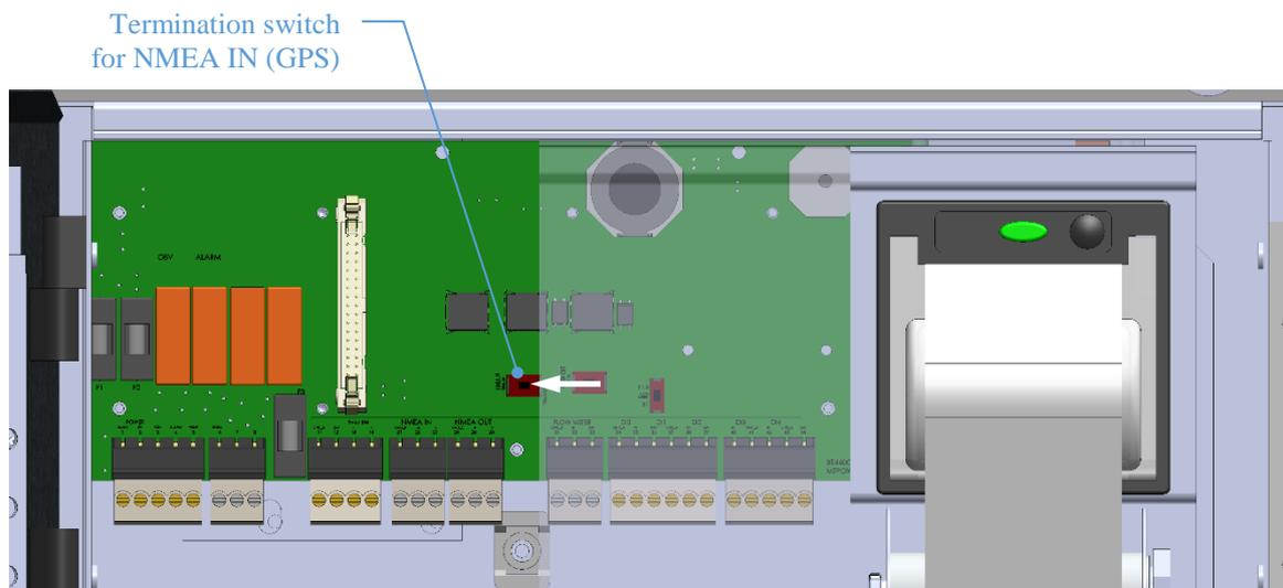
Figure 26. RS-422 termination enabled (switch set to the left).
