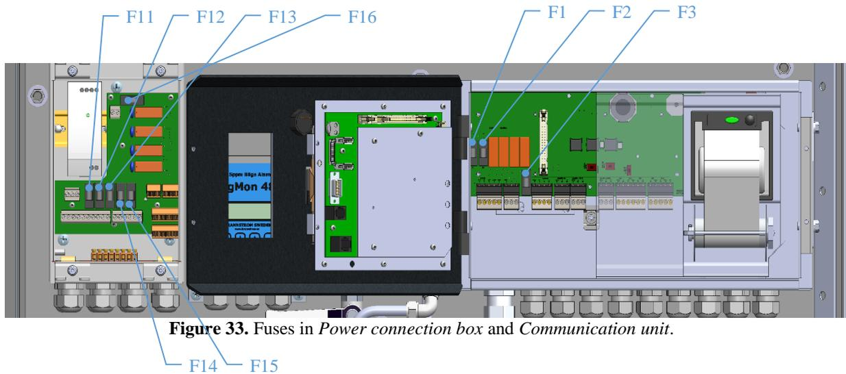
Figure 33. Fuses in Power connection box and Communication unit.
