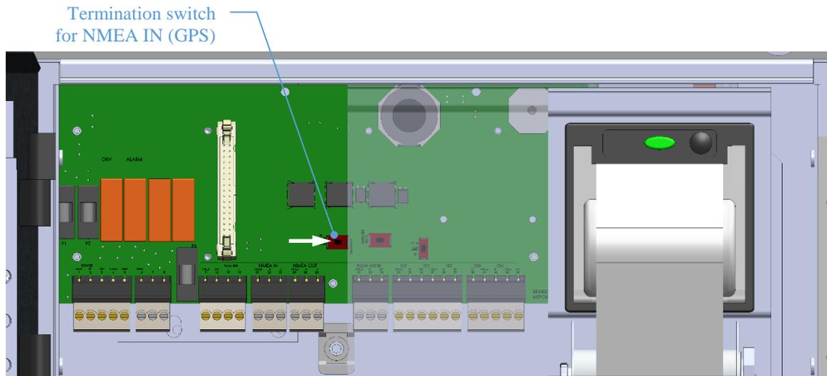
Figure 25. RS-422 termination disabled (switch set to the right).
