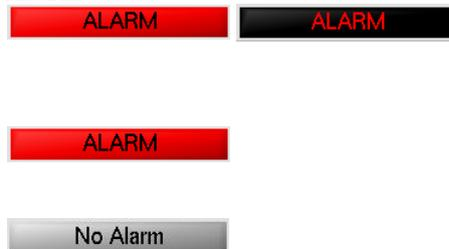
At least one alarm is active. Flashing between red and black. The buzzer is sounding. The alarm relay is open circuit. The alarm relay is also open circuit when MasterTrack 588® is powered off.
