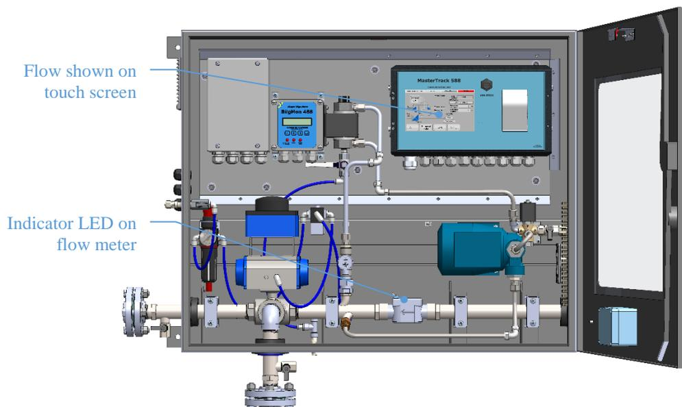
Figure 29. Flow shown on model B1.
