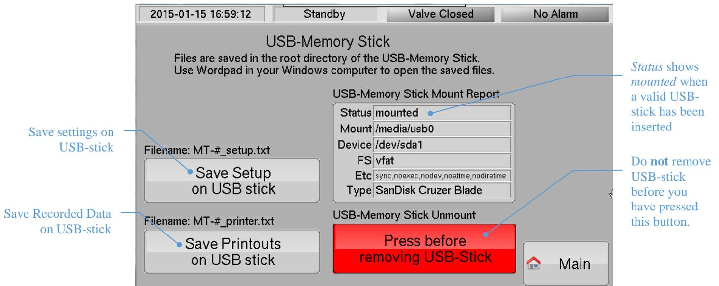
**Figure 24.** Screen as shown when a valid USB memory stick has been inserted.
