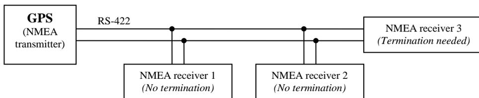
**Figure 27.** Termination should only be used by the last (or only) NMEA receiver.
