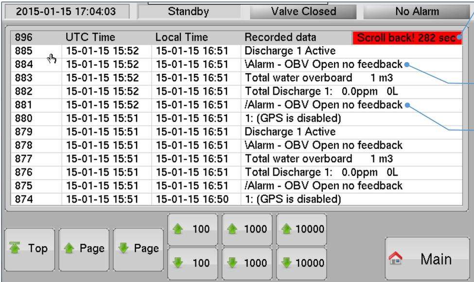
The screenshot shows the 'Recorded data' page with a table of events. The top status bar shows '2015-01-15 17:04:03', 'Standby', 'Valve Closed', and 'No Alarm'. A red box highlights 'Scroll back! 282 sec'. Annotations explain that new events appear at the top and older events are further down. It also notes that the alarm was cleared and then activated again.
