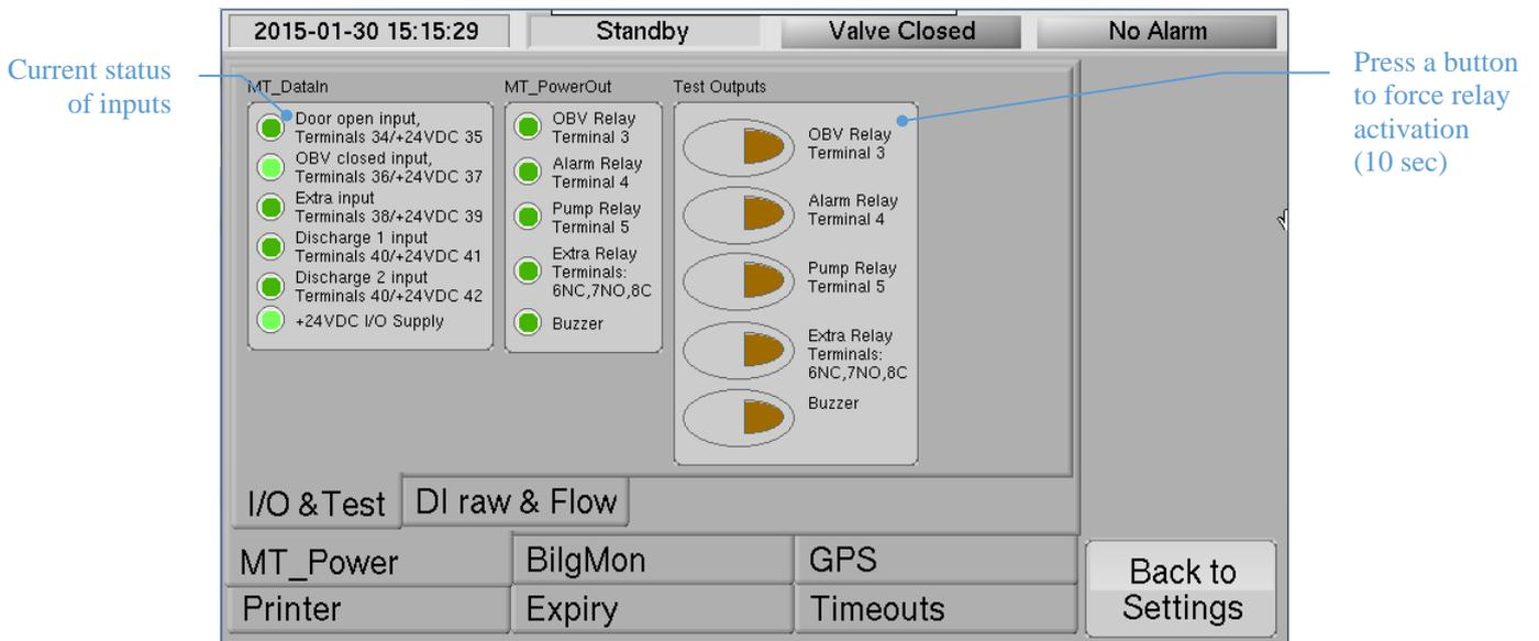
**Figure 23.** Settings – Advanced – MT\_Power – I/O & Test: Use this menu to see the state of the inputs and to test the relay outputs.
