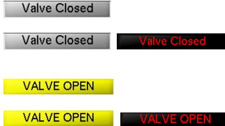
Overboard valve is closed (discharged water goes to sludge tank).
