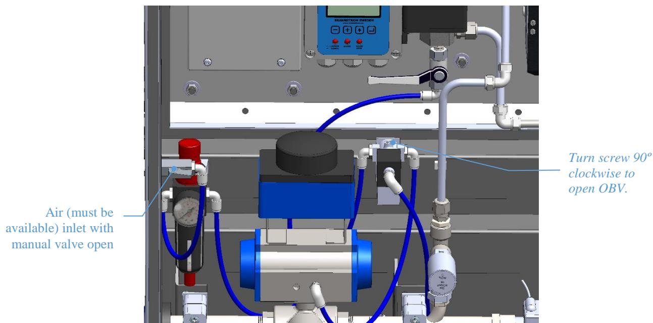
**Figure 28.** Turn screw to force OBV to open.
