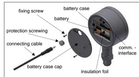
Fig. 3 Battery case and communication interface
