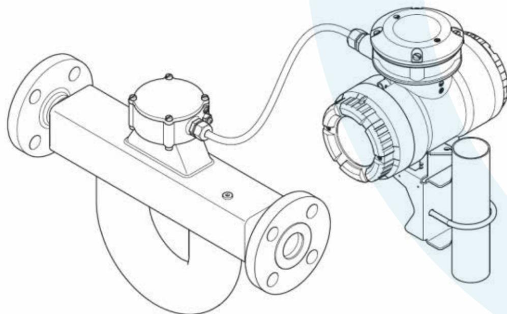
At zero flow, the oscillation of the 'legs' will be synchronized with both sensors registering the same pulse frequencies at the same time. When a flow is introduced through the sensor piping, the U-shaped sensor pipe will start to 'wobble' due to the Coriolis Effect, as the moving mass will 'delay' the upstream pulse. The two sensors will now experience an offset in the pulses, and the larger the offset the larger the flow is.
