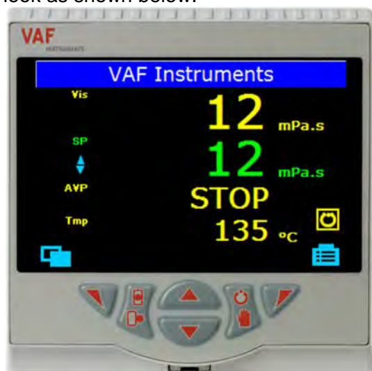
Figure 10 Dual channel controller in viscosity type mode, with relay output
