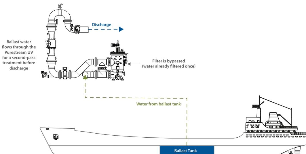
Purestream system is validated to operate at **minimum retention times** ( $\leq 24$  hours) following treatment of 100% of the maximum flow under difficult water conditions with UV transmittance as low as **40% UVT**.
